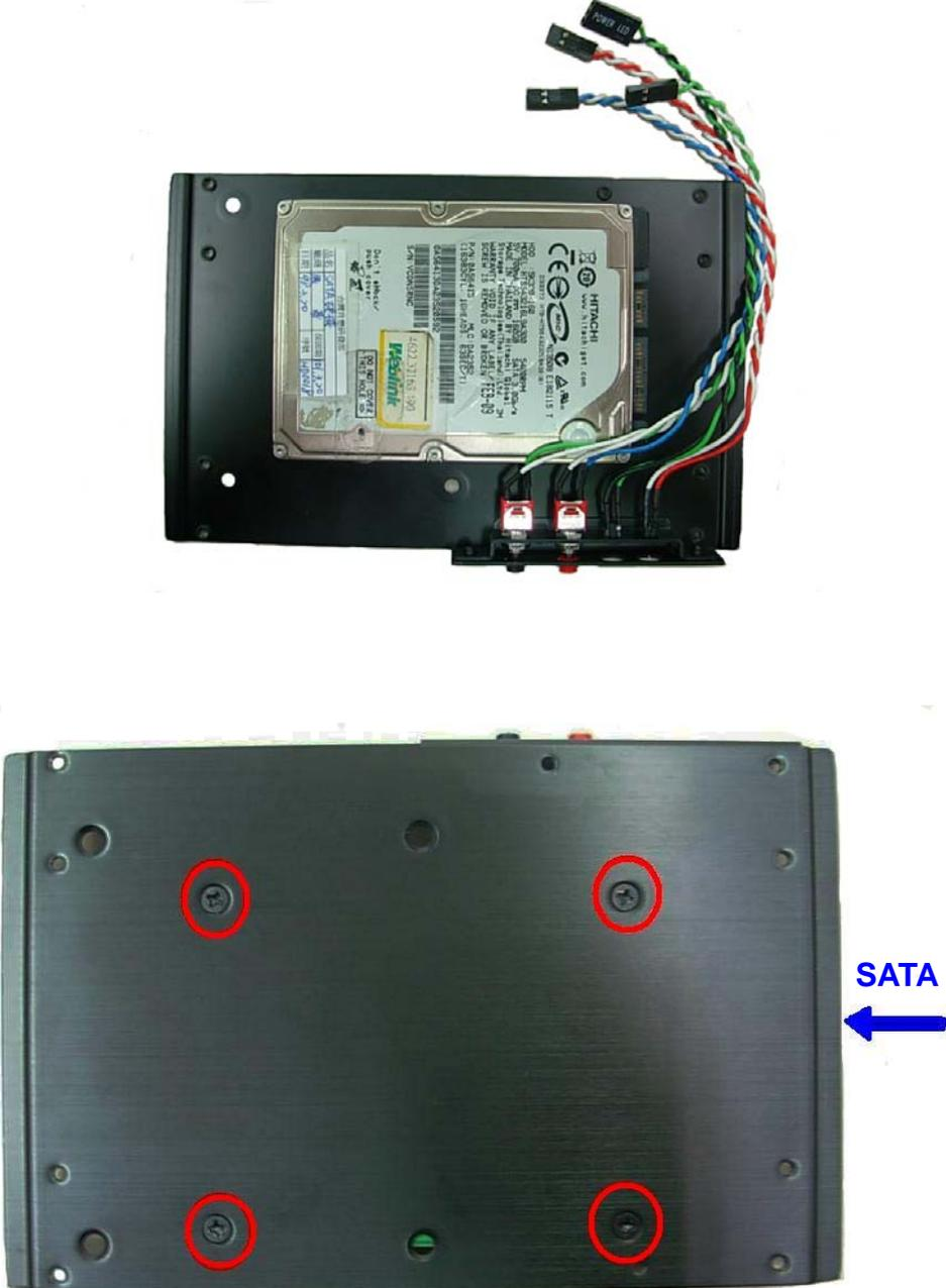
8. Connect the SATA and SATA power cable , power LED , HDD LED , reset bottom , power bottom cables.
