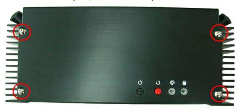
10. Lock the chassis feet screws.
