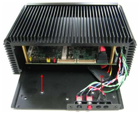
10. Lock the USB cable screws , put back the front panel , final lock the front panel screws.
