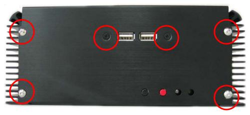
11. Lock the chassis feet screws.
