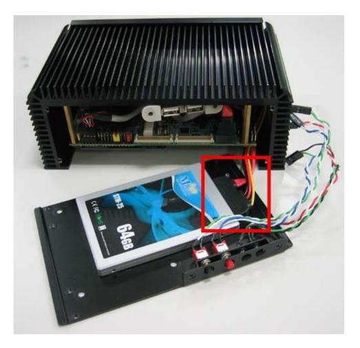
9. Connect the reset bottom , power LED , HDD LED , power bottom cables.
