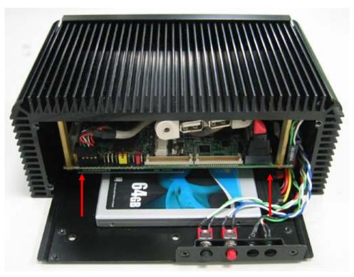
11. Lock the USB cable screws , put back the front panel , final lock the front panel screws.
