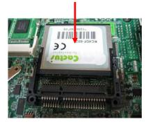
Installing the CFAST in the back of the board.
