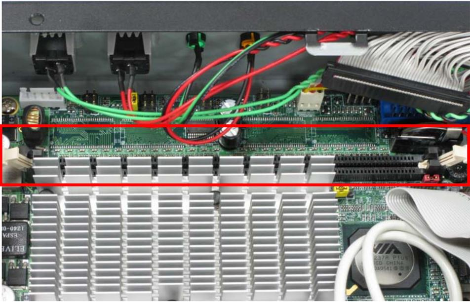
5. Press down the memory module then check DIMM holder hook well.
