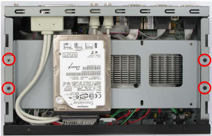
9. Push the Chassis shield towards the back then open it.
