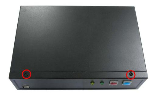
2. Push the Chassis shield towards the back then open it.
