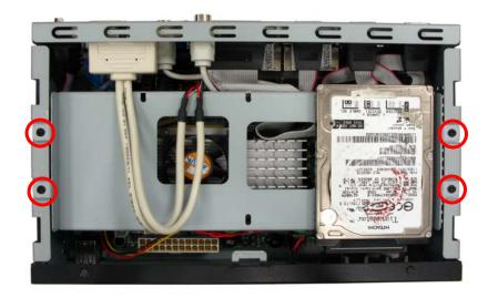
11. Push the Chassis shield towards the back then open it.
