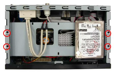
4. Turn the CPU cooler screws and then refer the motherboard manual page.17 to install the CPU.(After installing CPU, please turn the CPU FAN screws to tighten.)
