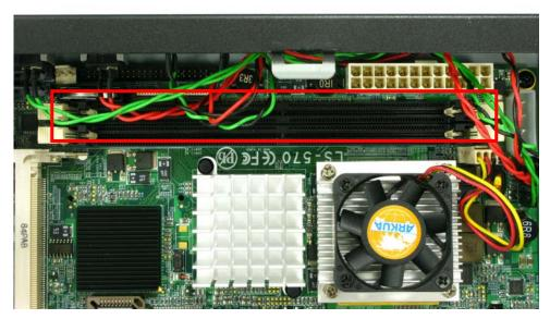
7. Press down the memory module then check DIMM holder hook well.
