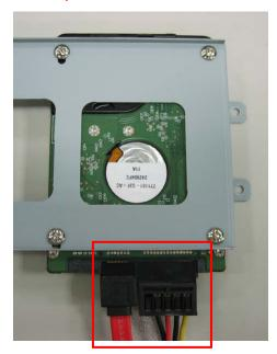
9. Screw on as indication of the picture below Turn the screws.
