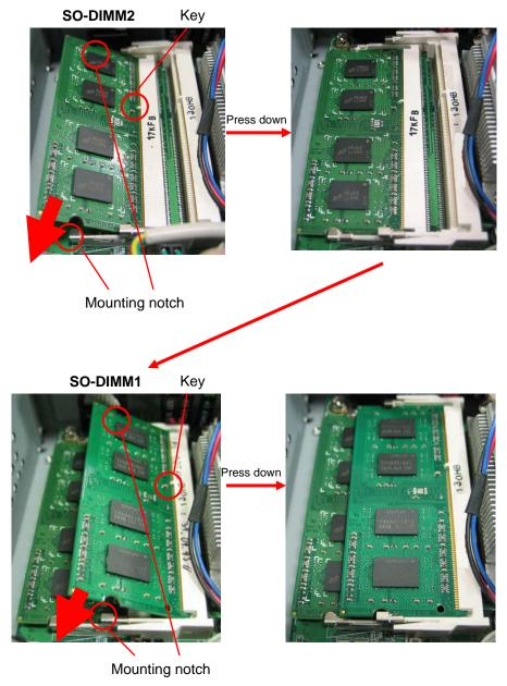
When you need to remove the memory, push outward on both sides of the latch.
