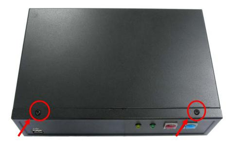
12. Turn the chassis shield screws with the Wall-mount brackets to tighten well.
