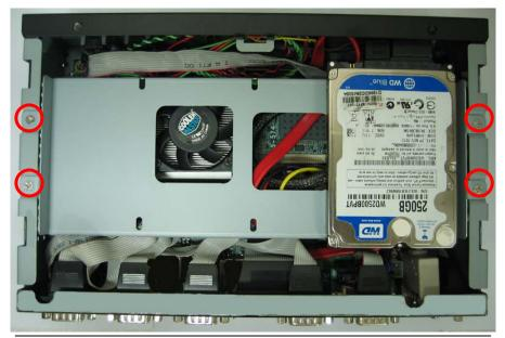
10. Push the Chassis shield towards the back then open it.
