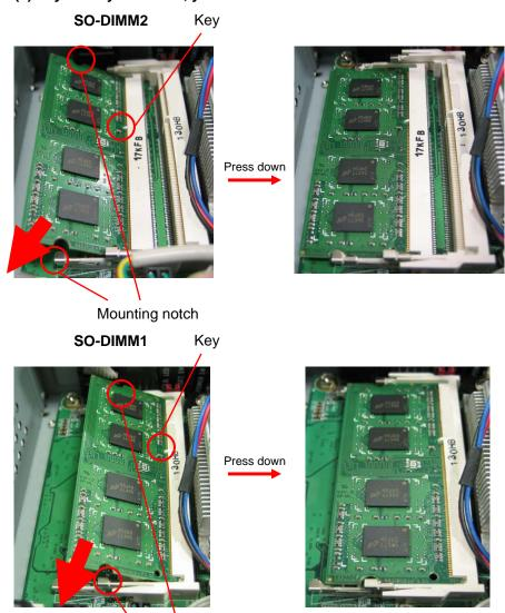
Mounting notch When you need to remove the memory, push outward on both sides of the latch.
