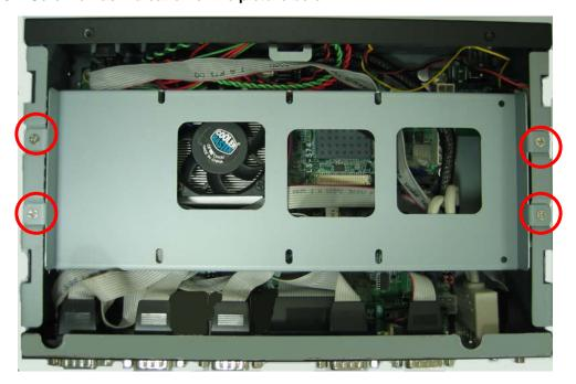
Turn the CPU cooler screws and then refer the motherboard manual page.15 to install the CPU.(After installing CPU, please turn the CPU FAN screws to tighten.)
