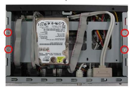
7. Push the Chassis shield towards the back then open it.
