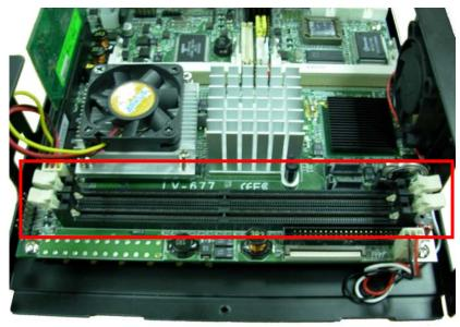
7. Press down the memory module then check dimm holder hook well.
