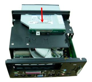
13. Turn the CD-ROM driver screws and IDE cable connects well.
