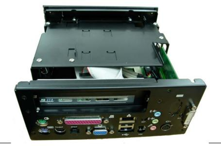
12. Take CD-ROM shield off . And insert CD-ROM drive from front panel to
