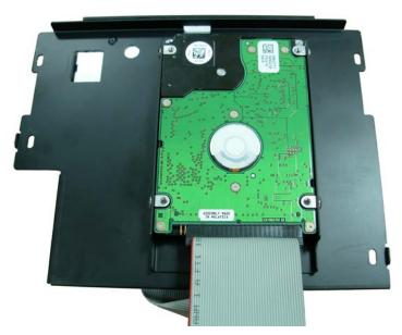
11. After install HD driver, Turn the CD-ROM holder and front panel screw well. (If you don't have CD-ROM driver please direct to step.14)
