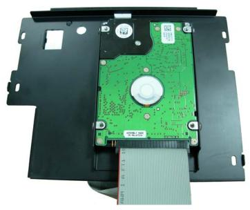
11. After install HD driver, Turn the CD-ROM holder and front panel screw well. (If you don't have CD-ROM driver please direct to step.14)
