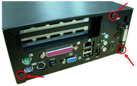
2. Push the Chassis shield towards the back then open it .
