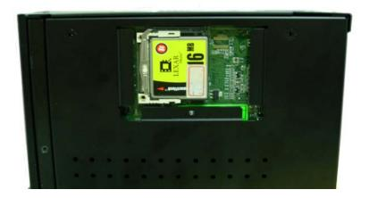
5. Close CF chassis shield and turn screw to tighten.
