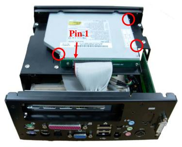
14. Turn the chassis shield screws to tighten well.
