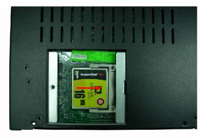
4. Close CF chassis shield and turn screw to tighten.
