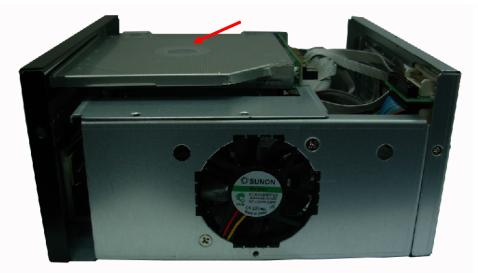
19. Turn the chassis shield screws to tighten well.
