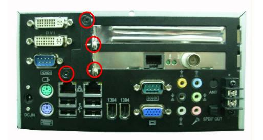
10. After install HD driver, Turn the CD-ROM holder and front panel screw well refer picture.
