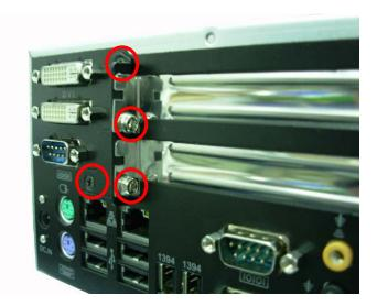
(B). You can install Riser-Card PCI-2P1 PCI card.
