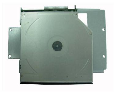
15. Find out the HD holder to install HD driver, it is under backside of the CD-ROM holder.
