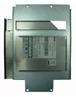
16. Put on HD driver into HD holder then turn the HD drive screws to tighten.(If you don't have HD drive please direct to step.18)
