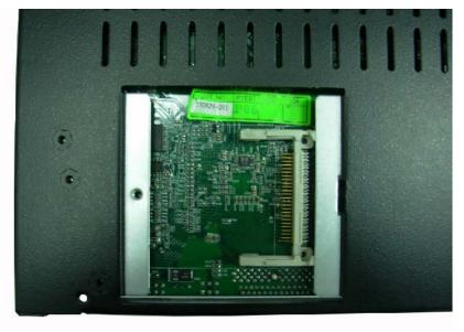
3. Follow the Idiot-proof design then insert the CF card, Check connected well.
