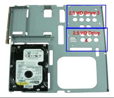
Put into HD driver and connect the cable well then turn the HD driver screws. (If you don't have HD driver, please direct to step 10)
