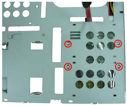
10. Before Install the CD-ROM. Turn the CD-ROM shield screws and take it off.
