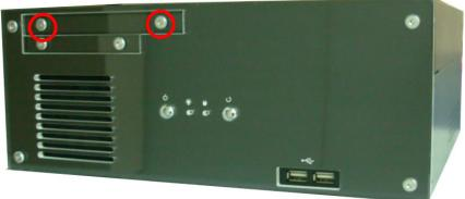
3. Open the CPU cover and refer the motherboard manual page.15 to install the CPU.
