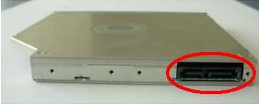
**10. Check the CD-ROM driver and SATA cable connects well, then connect the ATX output (4-pin).**
