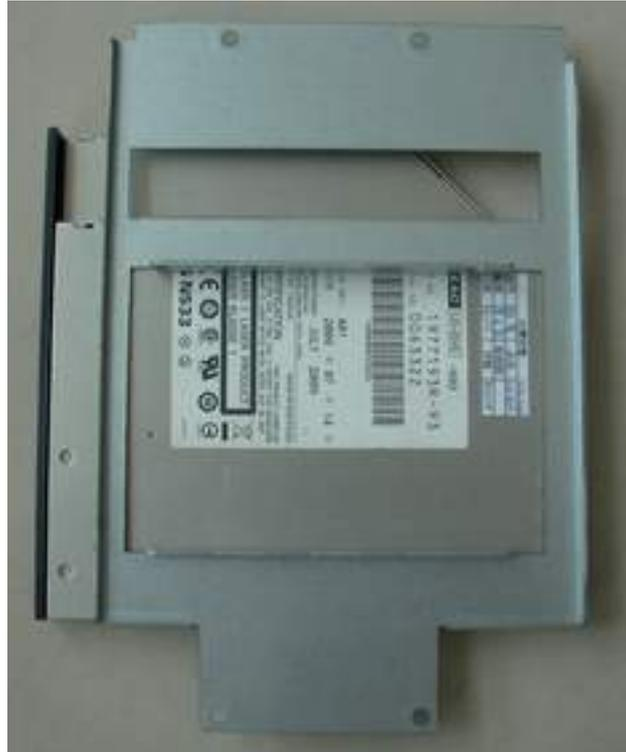
14. Put on HD driver into HD holder then turn the HD drive screws to tighten.
