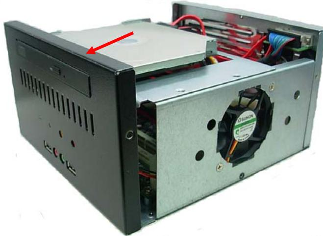
17. Turn the chassis shield screws to tighten well.
