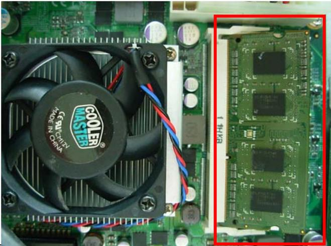
7. Press down the memory module then check dimm holder hook well.
