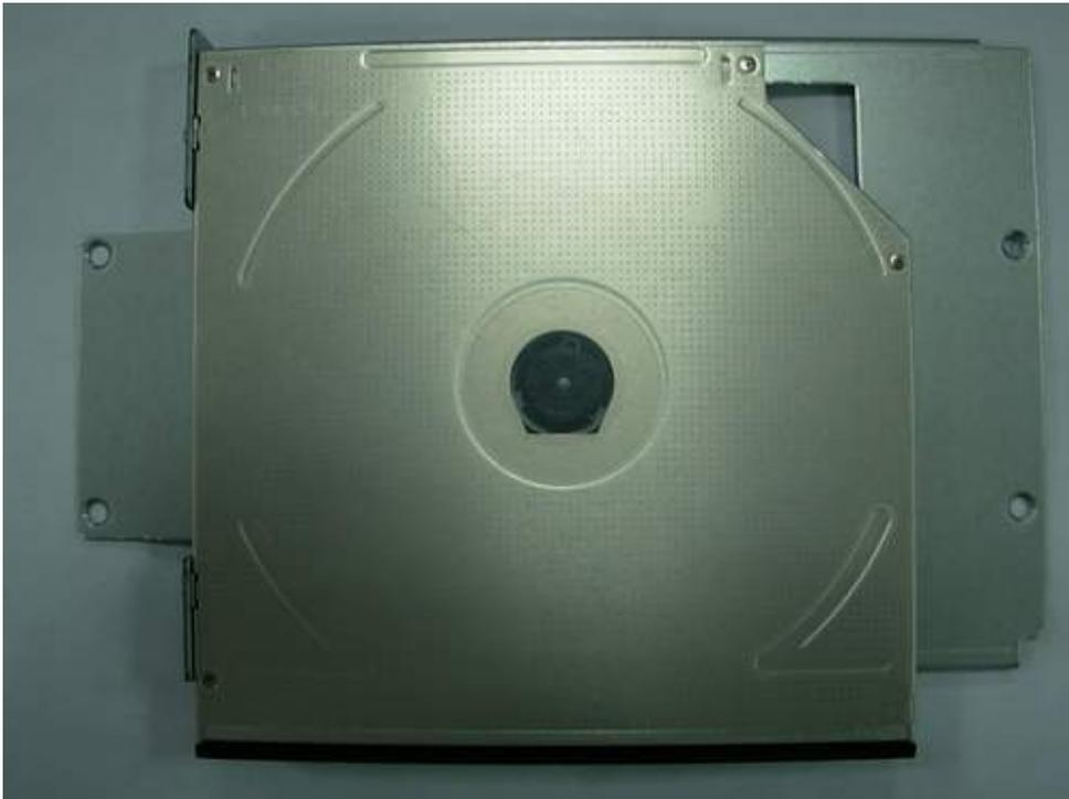
14. Put on HD driver into HD holder then turn the HD drive screws to tighten.
