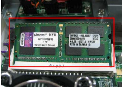
4. Press down the memory module then check dimm holder hook well.
