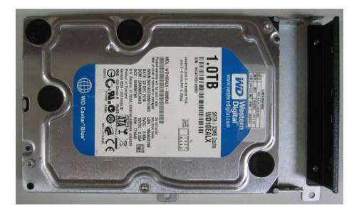
15. Screw the HDD by flat head screws by one way of (1) and (2).
