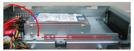
13. Screw back the HDD holder. (Direct to step 19.)
