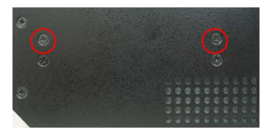
19. Push back the Chassis shield towards and screws.
