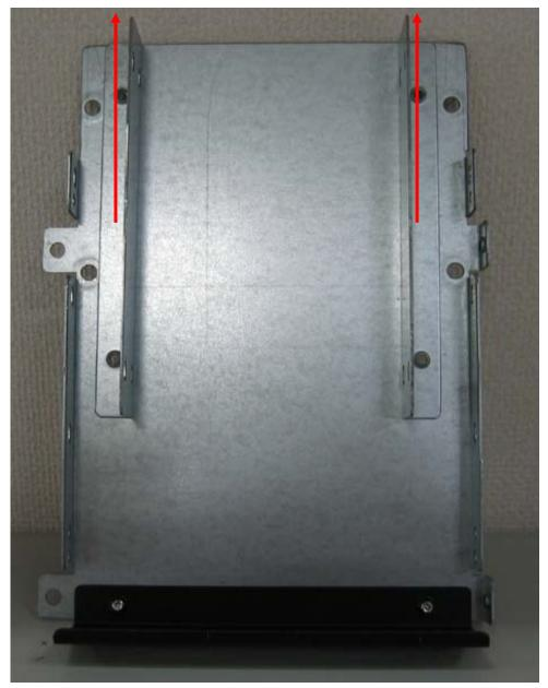
9. Take 2.5 inch HDD connect these two small HDD holders by screws, at most can use two. (Use 3.5 inch HDD please direct to step 14.)
