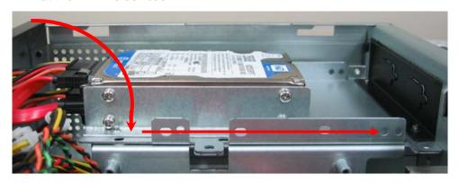
13. Screw back the HDD holder. (Direct to step 19.)
