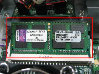
4. Press down the memory module then check dimm holder hook well.
