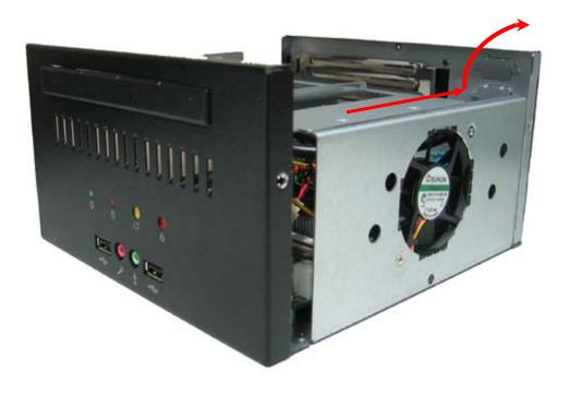
5. Open the Dimm holder then check the pin number to match the socket side well before installing memory module. (It has two slots to choice, or use both of them.)
