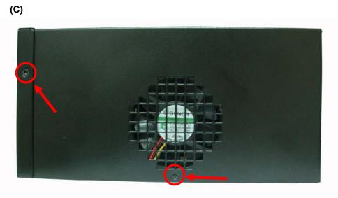
2. Push the Chassis shield towards the back then open it.
