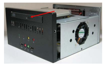
17. Turn the chassis shield screws to tighten well.
