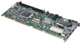
1 x FS-A79 PICMG 1.3 Full-size CPU Card motherboard
