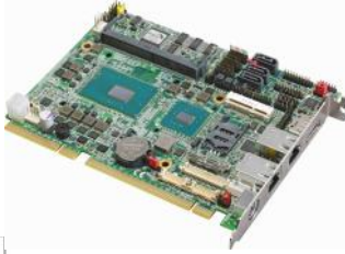
1 x HE-B72 PICMG 1.3 Half-size CPU Card (include Cooler Fan)
