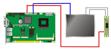
After setup the devices well, you need to select the LCD panel type in the BIOS.
