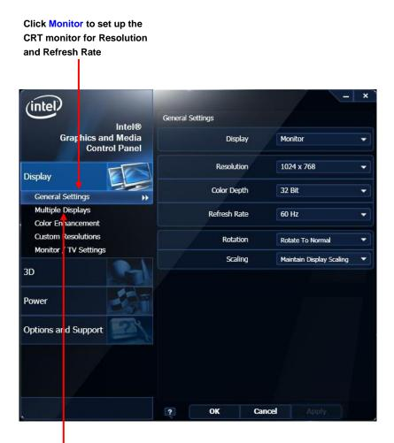
Click Intel® Dual Display Clone to set up the dual display mode as same screen
