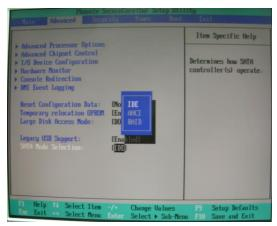
This option can let you select whether the Serial ATA hard drives would work under normal IDE mode or RAID mode. The RAID mode need more than one HDD is applied.
