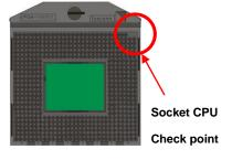
1. Use a slotted screwdrive to unlock the CPU socket 2. Follow the pin direction to install the processor on the socket
