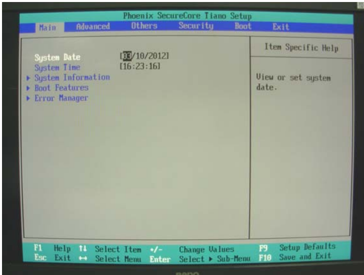
Figure 4-1 CMOS Setup Utility Main Screen
