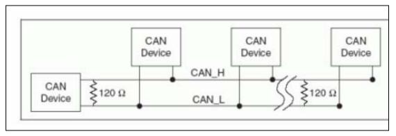
Figure 30 High-Speed CAN Networking
