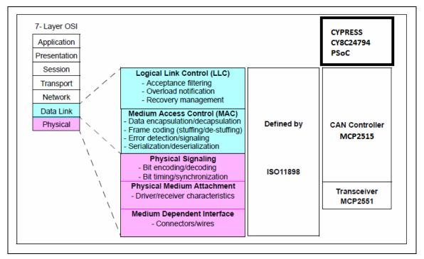
Figure 9 MPX-2515 ISO/OSI Reference Model
