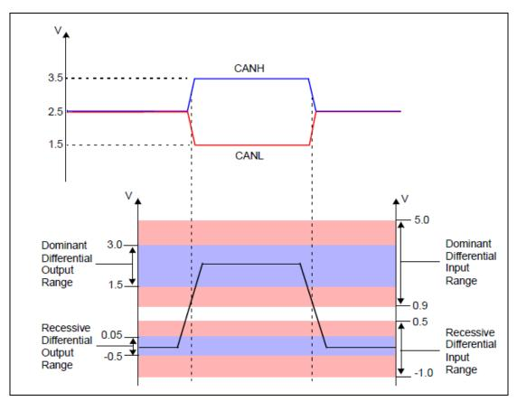
Figure 11 CAN Differential Bus
