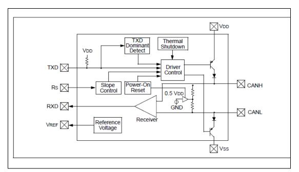
Figure 8 MCP2551 Block Diagram
