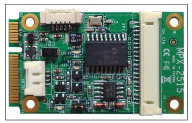
Figure 1 MPX-2515 CAN 2.0B USB Card
