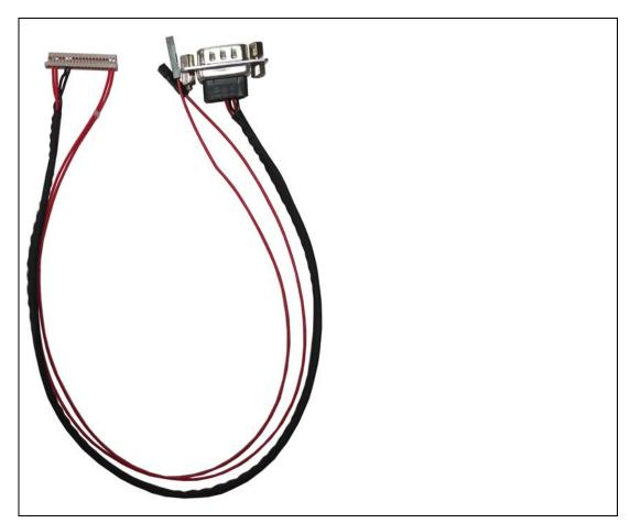
Figure 31 MPX-2515 Card Connects to CAN bus
