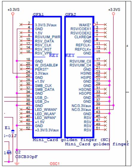
The following figure shows the I/O pins definitions of MPX-2515 CAN 2.0B USB card.
