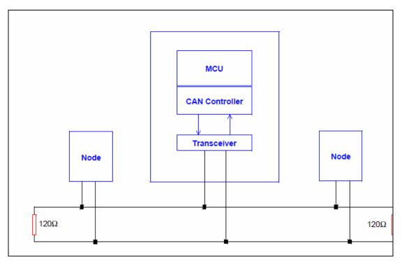
Figure 10 CAN Node on Bus
