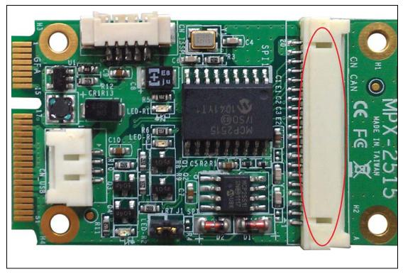
Figure 18 MPX-2515 CN\_CAN Connector
