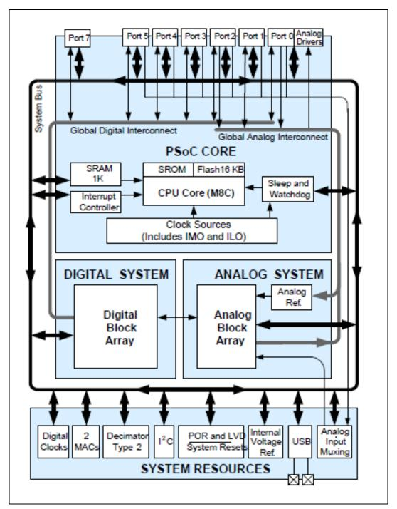
Figure 3 CY8C24794 Block Diagram
