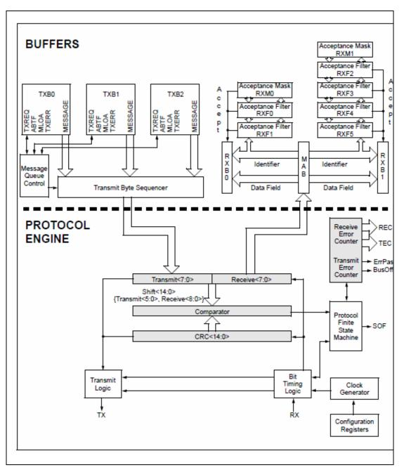
Figure 5 MCP2515 Buffers and Protocol Engine Blcok Diagram
