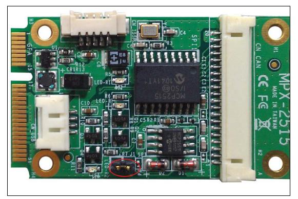
Figure 17 MPX-2515 Line Termination Jumper
