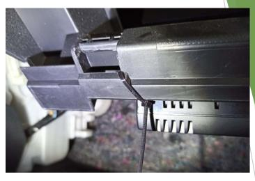
4. Fix it with cable ties behind glove compartment
